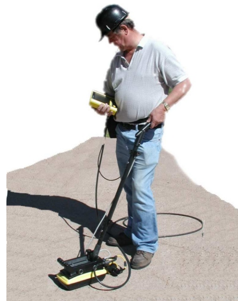
Figure 3. GPR equipment in use
