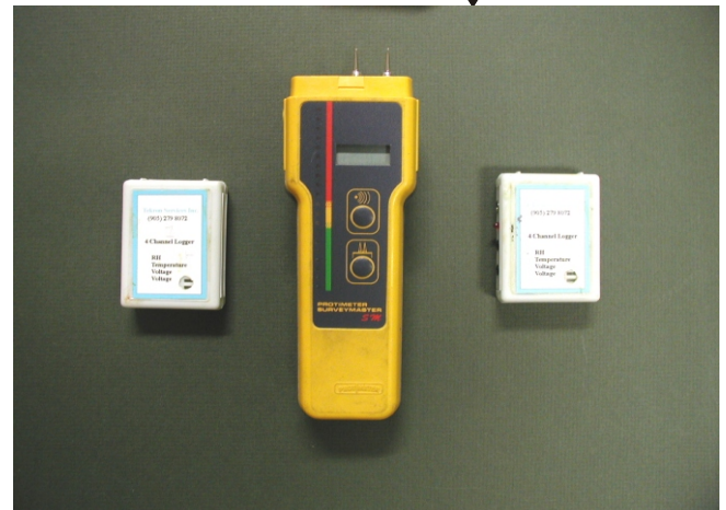
Protimeter and two temperature and humidity loggers
