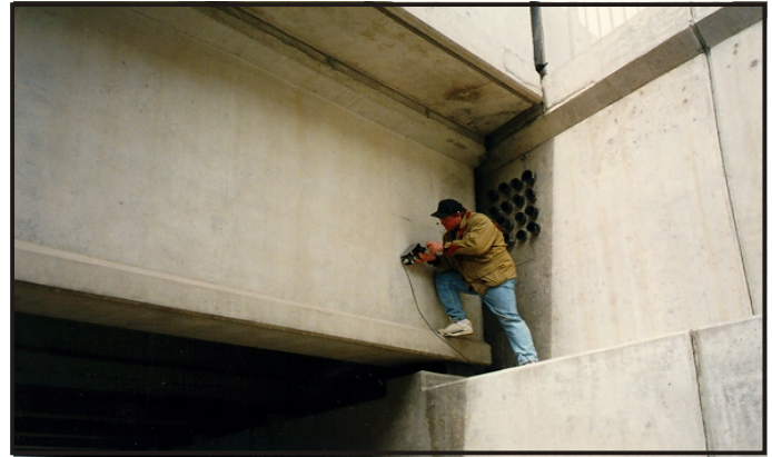
Testing Post-Tensioned Ducts with Impact-Echo Equipment
