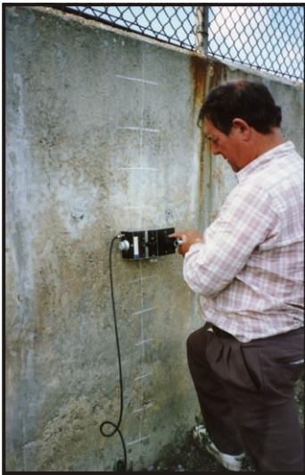
Testing retaining wall for internal cracking
